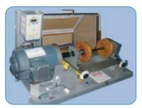
Considerable time shall be dedicated to hands-on practical sessions, taking vibration data and simulating machinery faults including unbalance, misaligment, losseness, bent shaft, rubbing and bearing damage.
